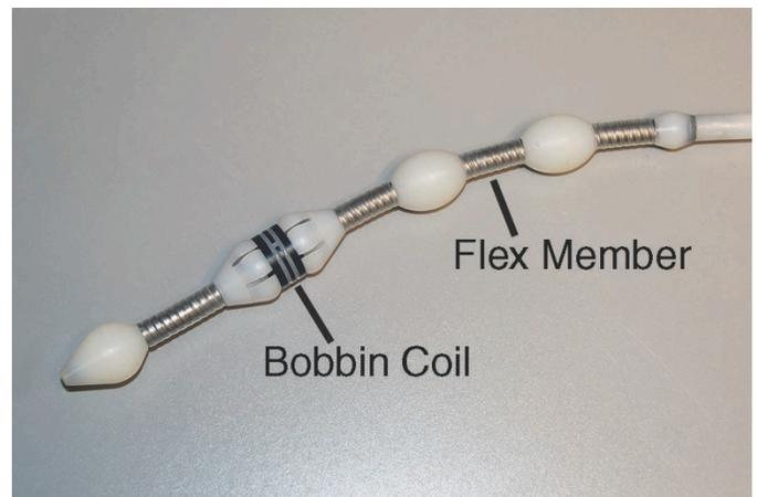
Figure 4. Flexible bobbin coil design that can negotiate U-bend tubes. (Photo Courtesy of Conco Services Corp.)
