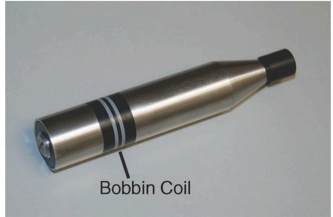
Figure 3. Standard issue barnacle scraper style bobbin coil in a self comparison differential coil arrangement. This can be configured to run in the external reference mode simultaneously with the self comparison mode. (Photo Courtesy of Conco Services Corp.)
