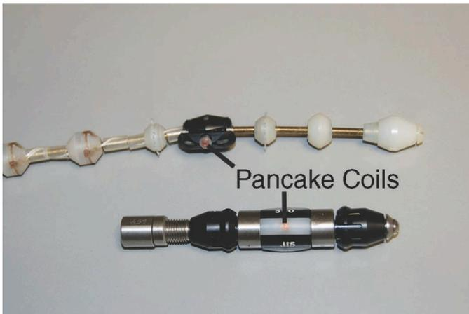
Figure 2. Probe coils mounted on a fixture to spin the coil inside of a tube to provide a focused surface scan. (Photo Courtesy of Conco Services Corp.)
