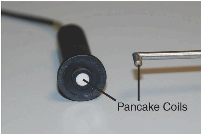
Figure 1. Probe coils in an absolute arrangement used for surface scanning. (Photo Courtesy of Conco Services Corp.)
